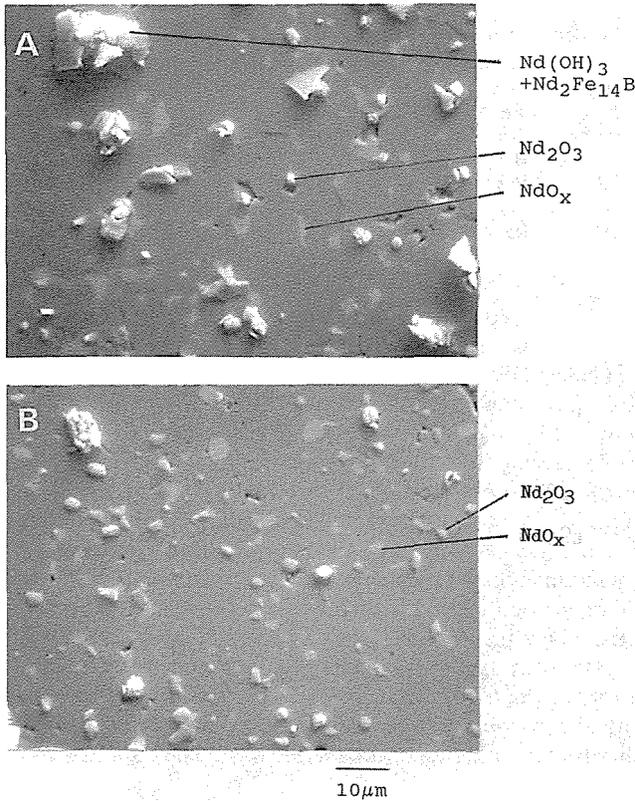
FIG. 6—SEM micrographs of Specimens A and B after polishing, back-scattered image (BSI), X1000.
