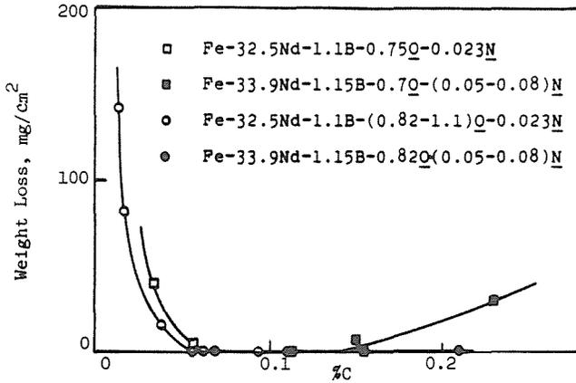
FIG. 2—Weight loss of Nd-Fe-B magnets after exposure in autoclave at 5 to 10 psig (35 to 69 kPa) for 96 h as a function of C content.
