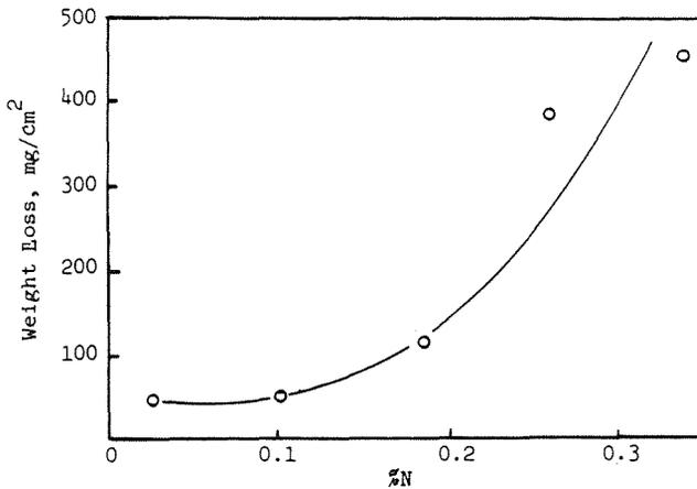
FIG. 5—Weight loss of Fe-34.2Nd-1.13B-0.55O-0.06C magnets after 40 h exposure in autoclave at 5 to 10 psig (35 to 69 kPa) as a function of N content.
