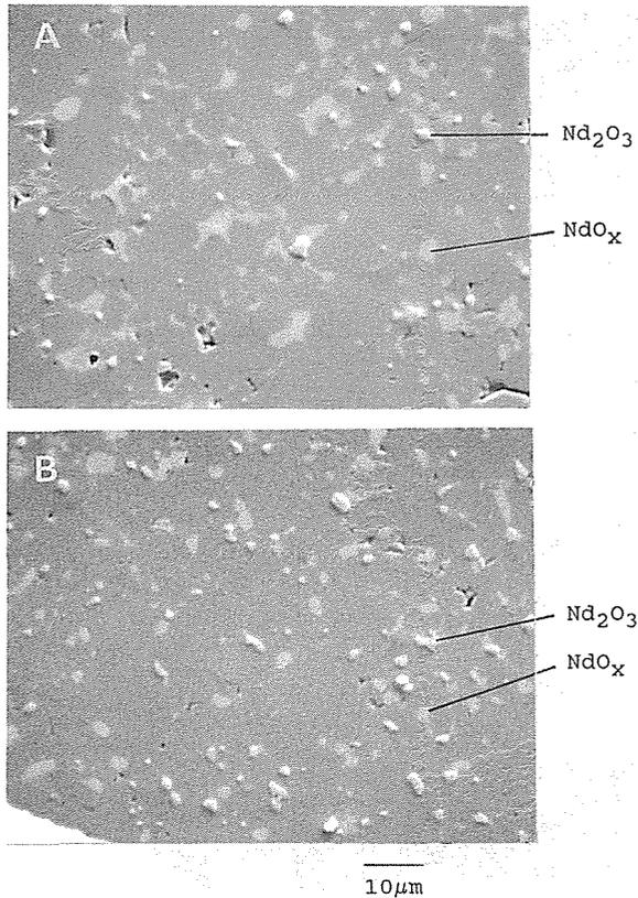
FIG. 7—SEM micrographs of Specimens A and B after 100-h exposure in air at room temperature, BSI, X1000.
