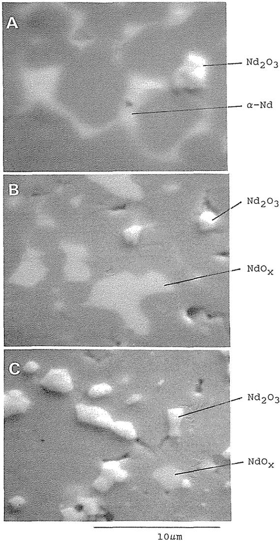
FIG. 8—SEM micrographs of Specimens C, D, and E, BSI, X5000.
