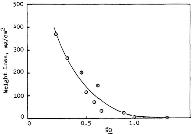
FIG. 4—Weight loss of Fe-33.5Nd-1.1B-0.1C-0.02N magnets after exposure in autoclave at 5 to 10 psig (35 to 69 kPa) for 96 h as a function of O content.
