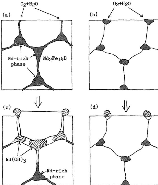
FIG. 9—Model for corrosion mechanism of Nd-Fe-B magnets in humid air: (a) Nd-Fe-B magnet with thick grain boundaries; (b) magnet with thin grain boundaries; (c) magnet (a) after exposure in humid air, and (d) magnet (b) after exposure in humid air.
