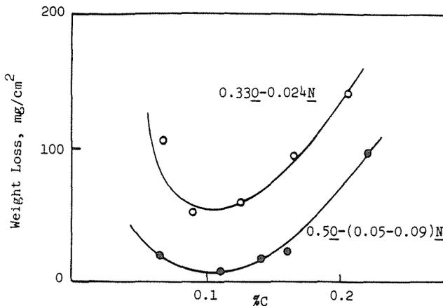
FIG. 1—Weight loss of Fe-33.9Nd-1.15B magnets after exposure in autoclave at 5 to 10 psig (35 to 69 kPa) for 40 h as a function of C, O, and N contents.
