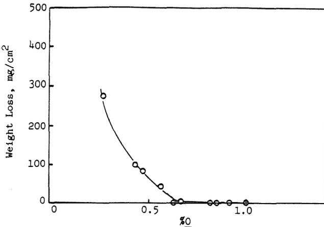
FIG. 3—Weight loss of Fe-33.5Nd-1.1B-0.1C-(0.05 to 0.15) N magnets after exposure in autoclave at 5 to 10 psig (35 to 69 kPa) for 96 h as a function of O content.
