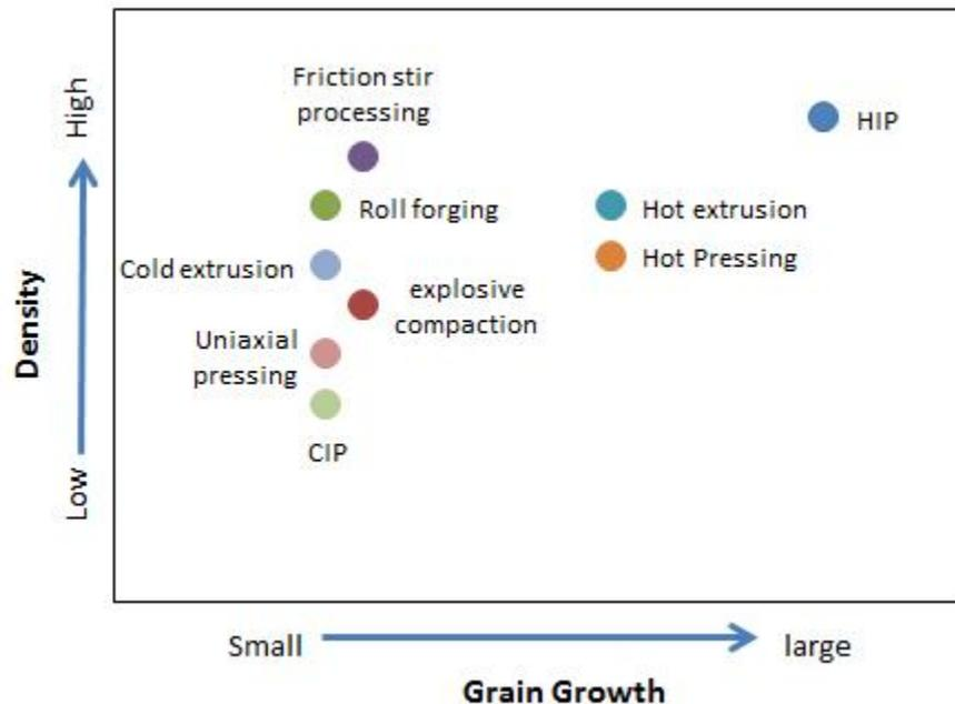
Figure 4 Evaluation of consolidation options regarding the impacts of consolidation processes on densification and grain structure stability of nanostructured materials.
