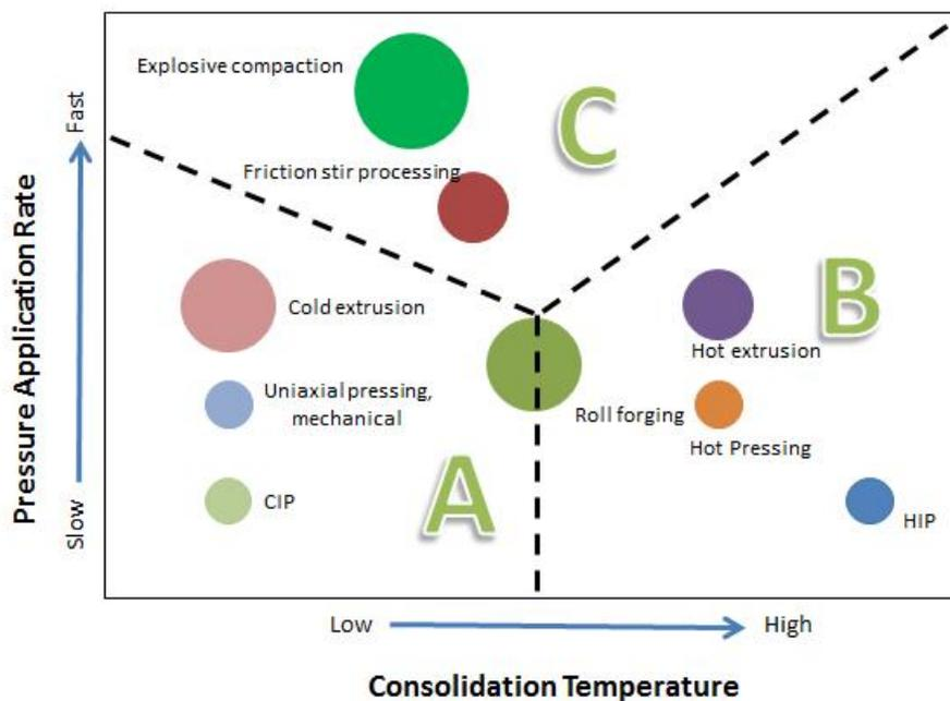
Figure 3 Consolidation process map: Bubble size represents magnitude of consolidation pressure; all data points are shown for illustration. A: insufficient for consolidation; B: microstructure unstable; C: potential for full density and stable microstructure.
