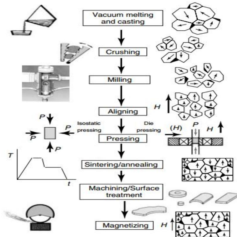
Figure 1 A typical process of manufacturing traditional energy critical permanent magnets.<sup>6</sup>
