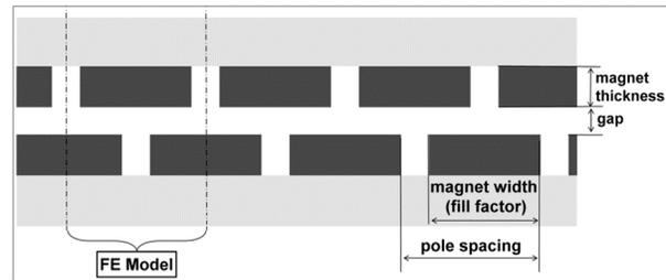
Fig. 7: Infinite planar coupling model
