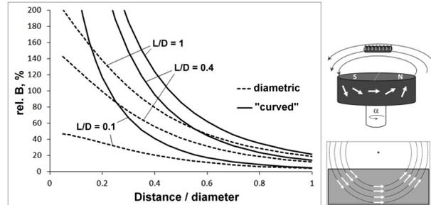
Fig. 3: Flux density on the axis of a cylindrical disc magnet of unit polarization and unit diameter.  $B$  = flux density in mT for a material with polarization 1T.  $L/D$  = ratio length/diameter.
