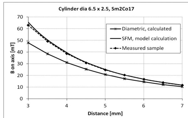
Fig. 4: Actual shaped field magnet example
