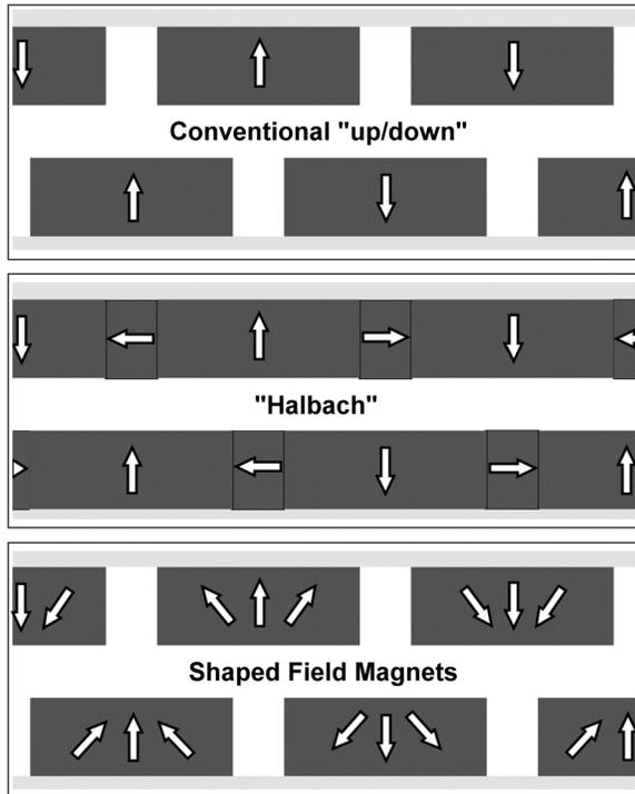
Fig. 5: Possible configurations for permanent magnet couplings.
