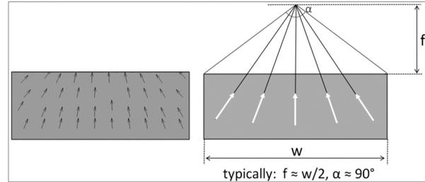
Fig. 6: Actual magnetization configuration and the approximation for modeling
