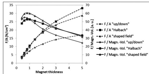
Fig. 8: Infinite planar coupling forces
