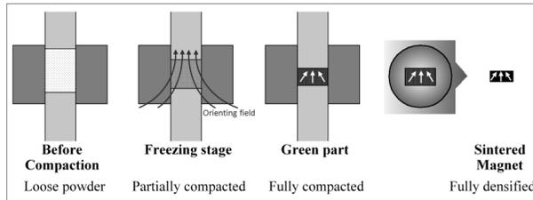
Fig. 2: Manufacturing process
